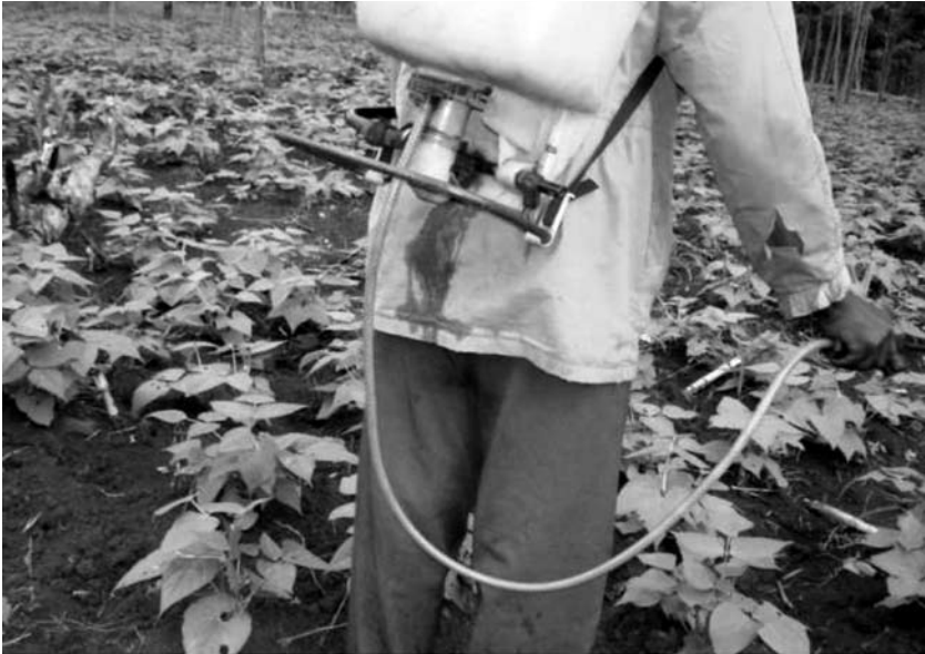
Pesticide leaking from equipment onto a producer spraying without wearing any protection, Tanzania (Photo: AGENDA, May 2006)
