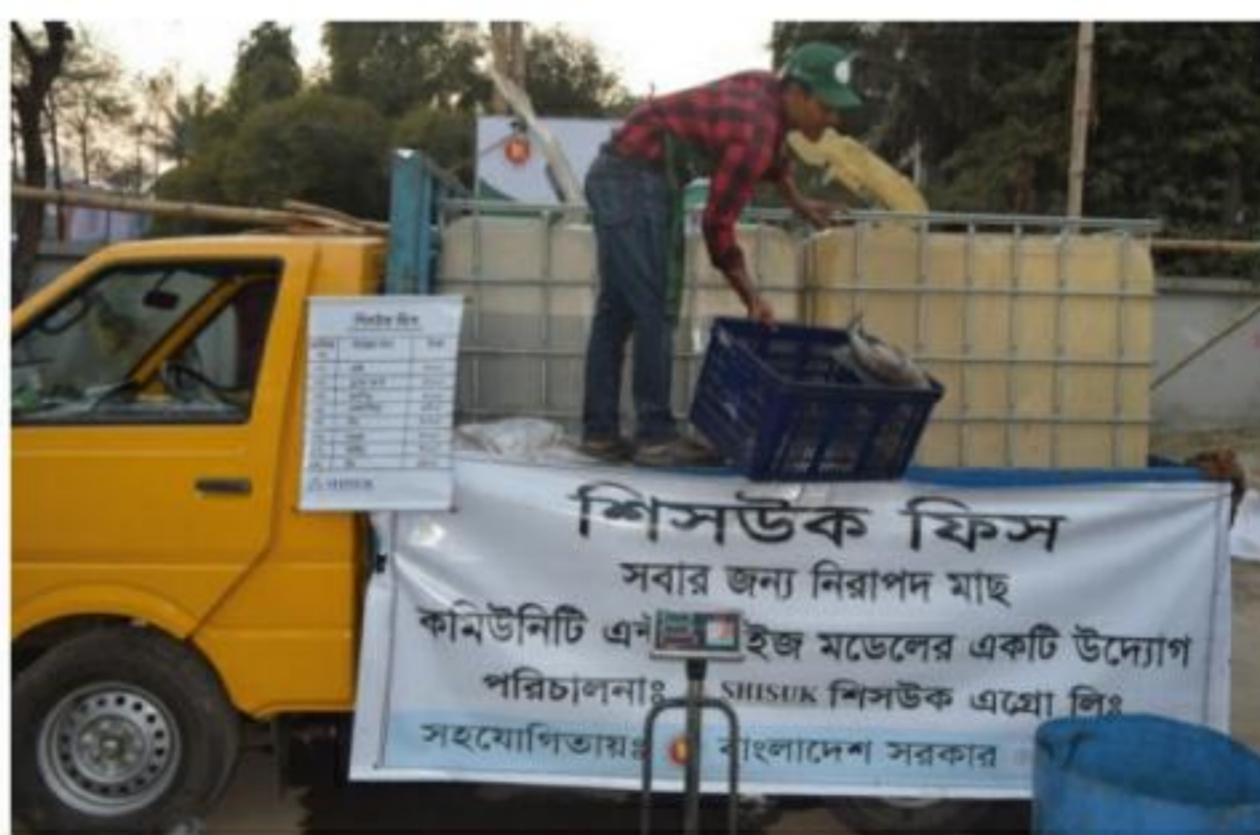
Local technic of selling live fish using water tank on the pick-up van with Oxygen cylinder. Innovation possible for solar aero rotator.
